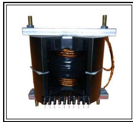
Figure 6.4: Designed ac-link inductor with 44 turns, 3 mm air-gap, and EPCOS Core PM87/70. Resulting inductance of 811 \mu H.
